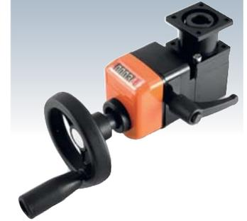
The RINV-OP65 is a flanged angular gearbox that, combined with a mechanical position indicator type "OP7" or an electronic position indicator type "EP7", allows to carry out a visualized adjustment, angular or linear, even if the shaft is in an uncomfortable position.
